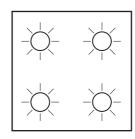
Each of the lamps may be turned on or off in order to configure a given signal. When the required combination is configured, the box is put on view so that it can be interpreted by the intended viewer.
